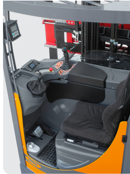
Mono-joystick (option) The mono-joystick includes all the machine hydraulic function.
