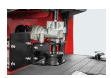
Electronic power steering system (for stand-up driving type tractor)
