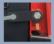
The locking device of the battery is provided with the safety protection function. Only if the locking device it rotated in place, the tractor can tray
