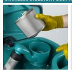
The vacuum motor is protected from impurities thanks to a stainless-steel filter, which is also easy to remove and clean.
