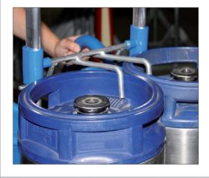
to secure KEG drums, height adjustable with hole rod
