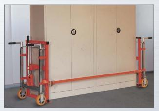
Hydraulic hoist unit with manual pump/relief valve, ball-bearing supported heavy-duty beams with soft polyurethane tyres and direct wheel steering with handles.
