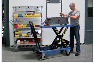
For assembling and working at an ergonomic height: The hydraulic pump is operated with the foot pedal. The lower-ing valve is operated with the hand lever.
