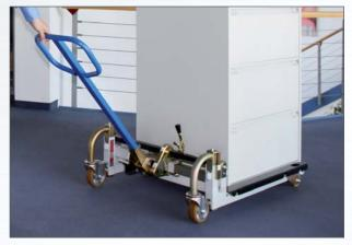
Using the multi- purpose lift truck, e.g cabinets can be lifted directly from the floor. It can be used for a wide range of tasks due to the laterally adjustable forks (400 - 825 mm).
