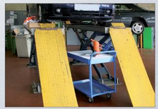
The ideal shop tool: material handling cart with drip tray and flush-mounted grating. This prevents damage, e.g. from dripping oil.
