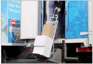
The retaining strap and the supporting skids allow the deepfreeze truck to be conveniently and safely pulled up or set down via the steps on the refrigerated truck.
