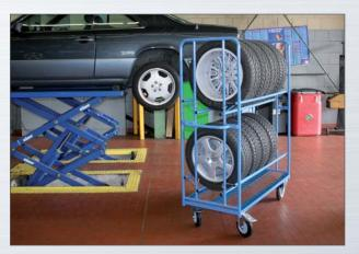
The angled supports on this special-purpose cart are suited for picking tyres and wheels, e.g. from the warehouse to the automobile shop.
