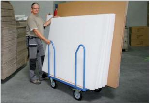
The side handle truck is used to conveniently move and maneuver bulky, heavy goods. The 750 mm high uprights are used as handles in this case.
