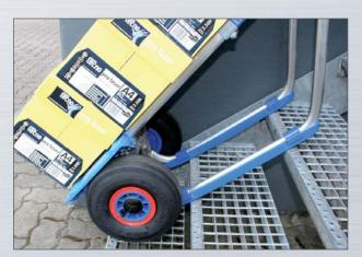
The anti-slip treads of the angled skids have an integrated red wear indicator to protect the structure. The clamp systems allows these to be replaced within seconds.
