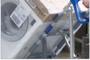
The many different protective profiles on multifunction hand trucks protect high-value and unpackaged goods against damage; also available as an accessory (see page 113).
