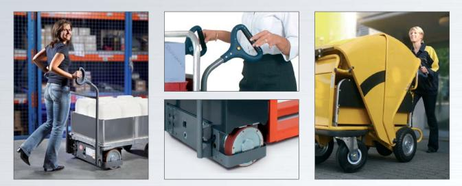
Thanks to the touch2move drive technology, logistics operations are optimised, and transporting heavy goods is not only more efficient, but also significantly safer. Simply by touching the sensor handles, the vehicle "obeys" the operator's natural movements, and automatically adapts to his/her walking speed. Heavy loads are moved safely and ergonomically without effort – and the operator needs neither a driving license nor any special training.
