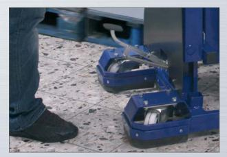
The lifting and lowering function is controlled by the foot pedal. The lift truck is maneuverable and therefore ideally used in commercial and warehouse buildings.
