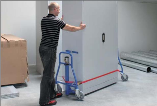
Mobile furniture hoist with manual lead screw crank for safe one-man transports of heavy cabinets, boxes, and other bulky goods.
