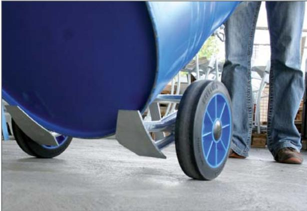
The unique triangular plates facilitate flexible uses since they permit the safe transport of a wide range of drum diameters.
