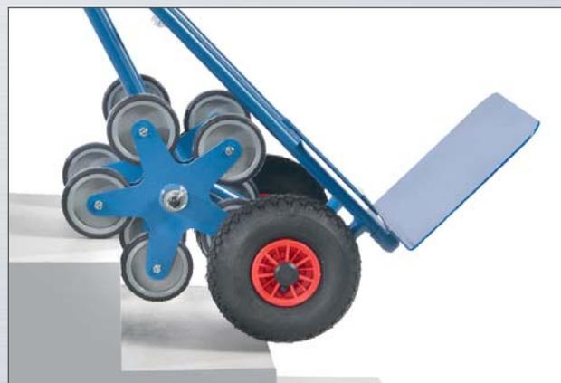
The stair hand truck with two pneumatic wheels and five-pronged wheel star provides advantages when moving on floor conditions in level areas with occasional stair travel.
