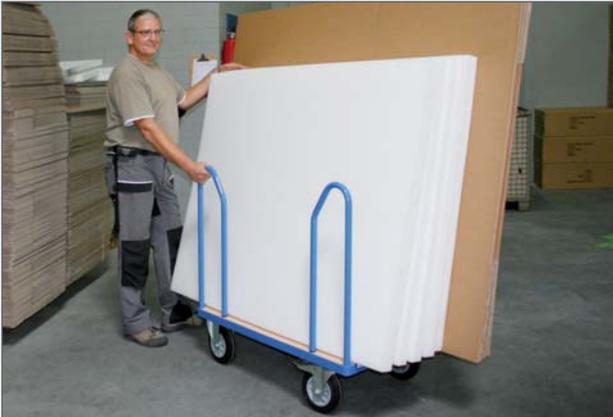
The side handle truck is used to conveniently move and maneuver bulky, heavy goods. The 750 mm high uprights are used as handles in this case.
