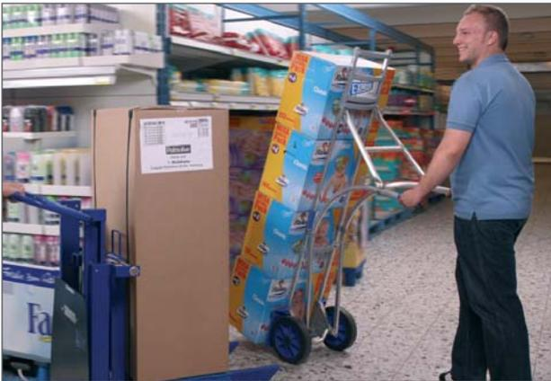
The warehouse hand trucks are characterized by their curved tube handle design. This allows carts with heavy loads to be easily tilted and moved.
