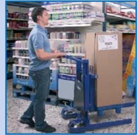
We recommend the combination pallet lifter with adjustable forks for transporting  $\frac{1}{4}$  and  $\frac{1}{2}$  pallets, and for picking orders from rolling containers.
