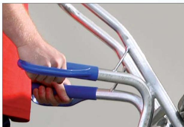
Frequently, it simply has to be steel: hot-dip galvanizing provides decades of corrosion protection without maintenance effort.
