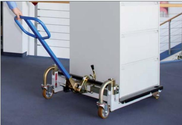
Using the multi- purpose lift truck, e.g cabinets can be lifted directly from the floor. It can be used for a wide range of tasks due to the laterally adjustable forks (400 – 825 mm).
