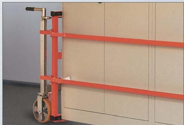
This is how it works: The footplate is pushed under the load, the integrated straps are tightened, the load is lifted with pump strokes and moved.
