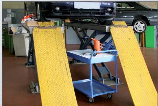
The ideal shop tool: material handling cart with drip tray and flush-mounted grating. This prevents damage, e.g. from dripping oil.
