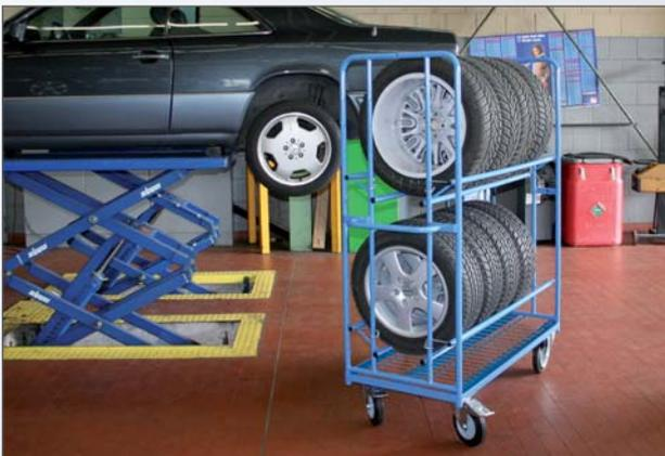
The angled supports on this special-purpose cart are suited for picking tyres and wheels, e.g. from the warehouse to the automobile shop.
