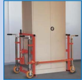
Mobile hydraulic hoist for transporting tools, control and steel cabinets, strong-boxes, heat pumps, boilers, machinery, housings, wet cells, boxes, etc.
