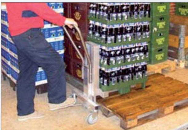
Hydraulic hoisting and lowering function to lift, handle, and transport quarter pallets, and for moving loads at floor level with a maximum payload of 250 kg.
