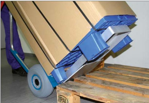
Using the pallet fork, ¼ pallets can be easily moved with a hand truck and effortlessly set down on a euro-pallet.
