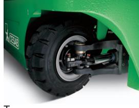
$T_{he \ new \ concept \ steering \ axle \ makes \ acute}$ steering angles possible and is mounted on silent blocks for improved operator comfort and quieter operation.
