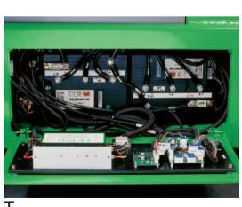
The electronic control unit, which is installed in the protected internal compartment, enables immediate access for programming and diagnostics. The truck performance characteristics can be adjusted to suit the working application and individual drivers needs.
