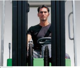
he cenTAURO range is available with new-concept 2 or 3 stage masts. The high visibility masts offer excellent visibility thanks to the placing of the lifting cylinders, in line with the mast profiles.
