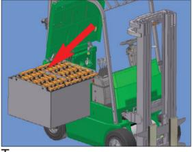
he optional lateral battery extraction allows battery change times to be minimised, optimising the truck's productivity.
