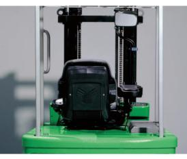
he ergonomic cab features the highest standards in operator comfort, safety and ease of access. The proportional electronic controls integrated in the new (optional) armrest enable the operator to manage all the hydraulic functions by simply moving the Mini-Joystick or Fingertips levers.
