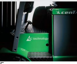
Excellent access to the driving seat, assisted by the large, conveniently located step with non-slip knurled aluminium tread.
