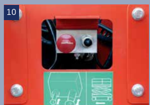
Manual release valve: When the machine doesn't work, you can push the machine after pressing this valve.
