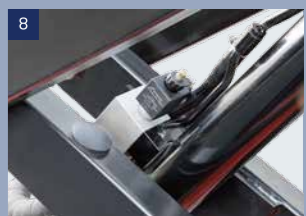
Explosion proof valve: To prevent the platform falling when the oil tube is leaking.
